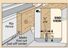
**Groove.** To cut the centered grooves, make the first cut, then flip the workpiece and make the second cut.
