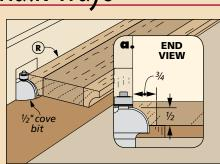
**Cove Molding.** With a cove bit in the router table, rout the molding in two passes to avoid tearout.
