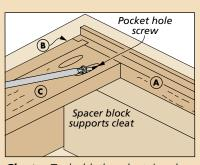
**Cleats.** To hold the cleat in place while driving the screws, I cut a spacer block from a piece of scrap.
