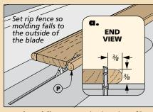
**Bead Molding.** Rout the bead profile on an extra-wide blank. Then rip the strips of molding free at the table saw.
