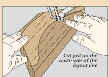
**Cut Out the Shape.** You can cut out the shape of the brackets using a scroll saw, jig saw, or band saw.
