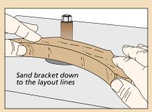
**Sanding.** A spindle sander works great for removing the saw marks and cleaning up the edges of the brackets.
