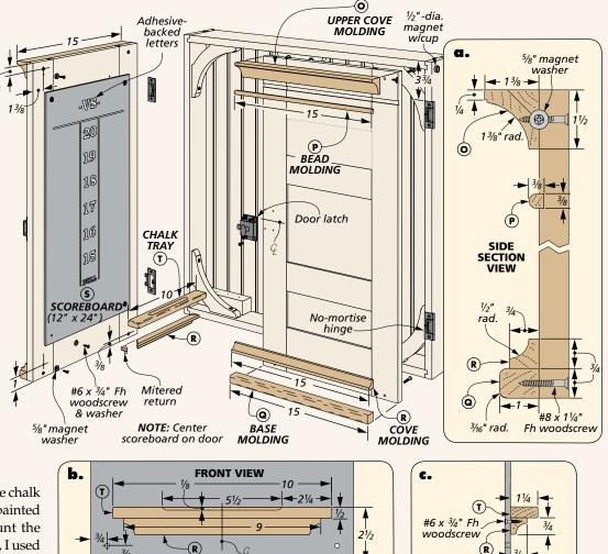
I used no-mortise hinges to hang the doors. There's nothing tough about installing these hinges. Just lay out the position on the cabinet sides and attach the hinges with screws. Put the door in position with shims to give it an even gap all around. Then screw the hinge to the door. After hanging the doors, I installed the latch with screws. Now, you can paint the beadboard back and screw it in place.
