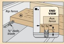
**Dadoes.** With a dado blade installed and an auxiliary fence on the miter gauge, use the rip fence to locate the dadoes.
