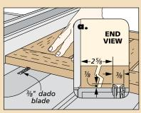
**Molding Channel.** Use a dado blade and the rip fence to cut the shallow groove for the bead molding.
