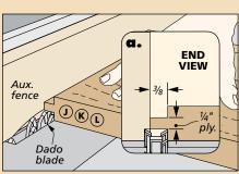
**Tongues.** Bury a wide dado blade in an auxiliary fence to cut the tongues. Sneak up on a snug fit to the grooves.
