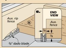
**Tongues.** Bury the dado blade in an auxiliary rip fence to cut the tongues. Sneak up on a snug fit to the dadoes.
