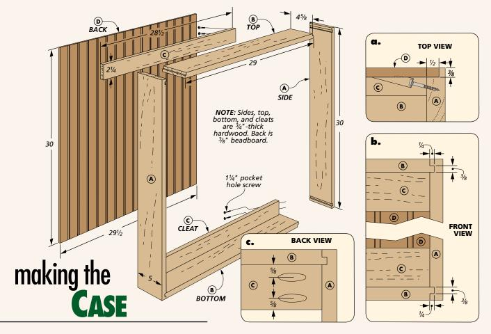
The basic case for the cabinet is pretty straightforward to build. The drawing above shows how I used tongue and dado joinery to connect the top and bottom to the sides. Cleats at the top and bottom of the case add strength to the joints. The addition of the beadboard back and corner brackets make the case rock-solid.
