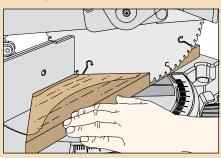
**Start with the Miters.** After tracing the pattern for the bracket on an oversize blank, miter both ends.
