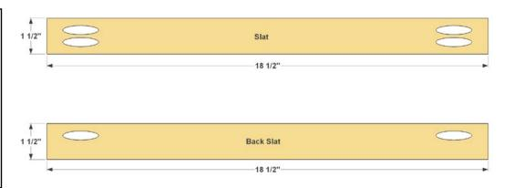
Step 5: Add the top shelf assembly by attaching five Slats and one Back Slat as shown using 1 1/4" fine-thread pocket hole screws. It's easiest if you attach the front-most Slat, and the Back Slat, and then space the remaining Slats evenly in between them.
