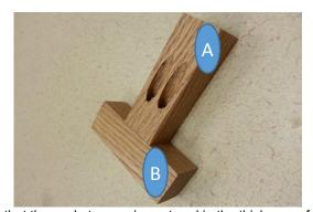
Note: Using the recommendations shown ensures that the pocket screw is centered in the thickness of the end of Part A where it joins Part B. When in doubt, test joints on scrap pieces. Screw Chart assumes Part B widht is 1-1/2" or greater.
