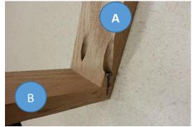
Note: Using the recommendations shown ensures that the pocket screw is centered in the thickness of the end of Part A where it joins Part B. When in doubt, test joints on scrap pieces.
