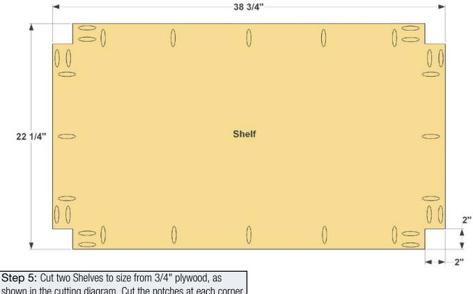
Step 5: Cut two Shelves to size from 3/4" plywood, as shown in the cutting diagram. Cut the notches at each corner using a jig saw. Then, with your pocket hole jig set up for 3/4" material, drill pocket holes in the Shelves, as shown.
