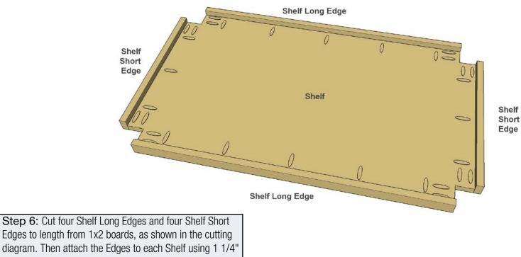
fine-thread pocket hole screws, as shown.
