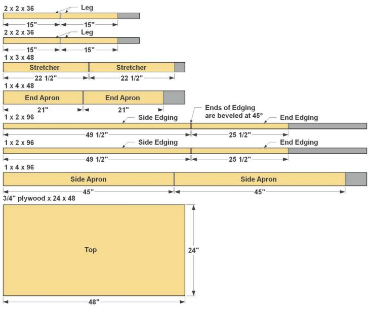
Step 1: Using the cutting diagram as a guide, cut two End Aprons to length from 1x4 boards. With your Kreg<sup>®</sup> Jig set up for 3/4" material, drill pocket holes in each End Apron, as shown.
