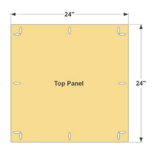
Step 11: Cut a Top Sheet, or have it cut for you, from a sheet of galvanized sheet metal.
