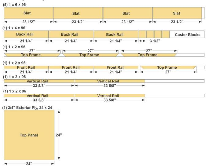
**Step 1:** Using the Cutting Diagram as a guide, cut twenty Slats to length from 1x6 boards.
