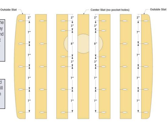
**Step 17:** Lay out a 6"-diameter hole in the top panel so that it's centered from side to side and 9" from one end.
