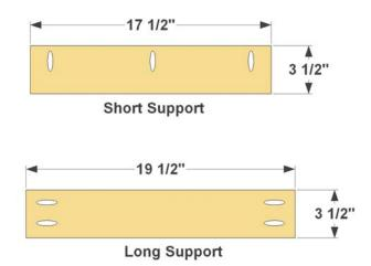
Step 12: Install the Supports in the base using 1-1/4"  $Kreg^{\otimes}$  Blue- $Kote^{TM}$  Screws.
