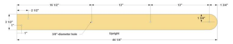
**Step 5:** Drill holes in the Uprights, as shown, for mounting bolts and for the threaded rods used to make the Ladder Rungs.
