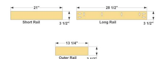
Step 3: Start base assembly by joining the Long Rails to the Short Rails using 1-1/4" Kreg<sup>®</sup> Blue-Kote<sup>™</sup> Screws. Then add two of the Outer Rails, as shown, using 1-1/4" flathead screws from the inside.
