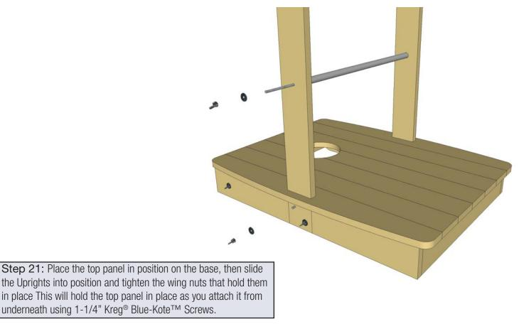
the Uprights into position and tighten the wing nuts that hold them in place This will hold the top panel in place as you attach it from underneath using 1-1/4" Kreg® Blue-Kote™ Screws.
