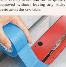
Apply the Tape. First, apply a piece of painter's tape across the top of the saw table a couple inches in front of the blade of the saw.
