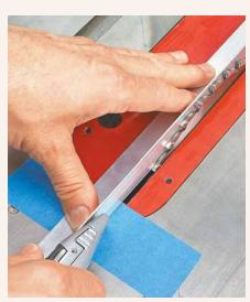
▲ Trim Along the Straightedge. With the straightedge lined up against the blade, cut a line through the tape, and remove the piece on the left.
