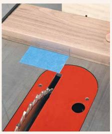
▲ Line Up the Cut. Then, all you need to do to make a quick and accurate cut is simply align the layout line on the workpiece with the left edge of the tape.
