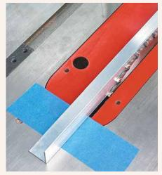
▲ Choose A Straightedge. The straightedge should have enough height and length to butt up against several teeth on the saw blade.
