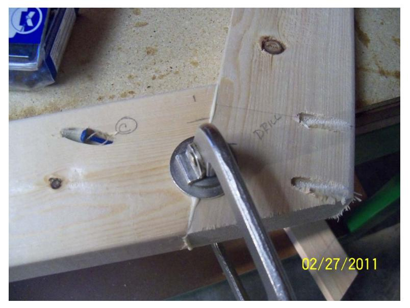
This was the final design. My question is; do you think I needed to place three screws in the joint and did they need to come in from both directions? I am changing the design of the picnic table leg assembly as it originally called for a 5/16" carriage bolt through the top brace and leg like is shown in the next slide. As you can see I glued the joint also. Thoughts?
