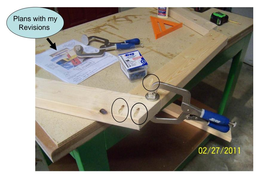
I am building a picnic table and converting some of the construction to pocket hole joinery.
