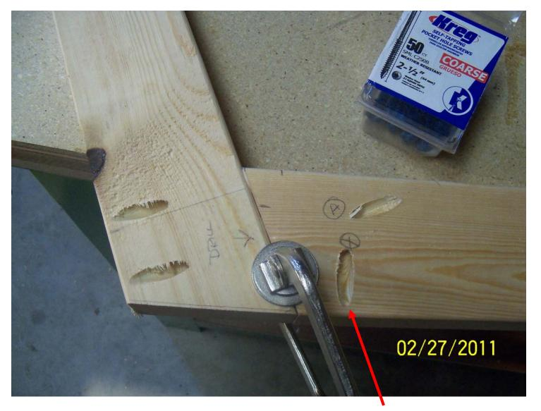
This hole was also drilled incorrectly!
