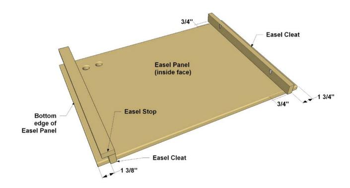
**Step 14:** Position the Easel Cleats on the inside face of the Easel Panel as shown. The lower Cleat should sit 1 3/8" from the lower edge of the Easel Panel, and the upper Cleat should sit 1 3/4" from the upper edge of the Easel Panel. The Cleats overhang 3/4" on each side. This creates gaps that reduce the chance of fingers getting pinched when sliding the Easel from side to side. Attach these two Cleats using glue and 1 1/4" coarse-thread pocket hole screws.
