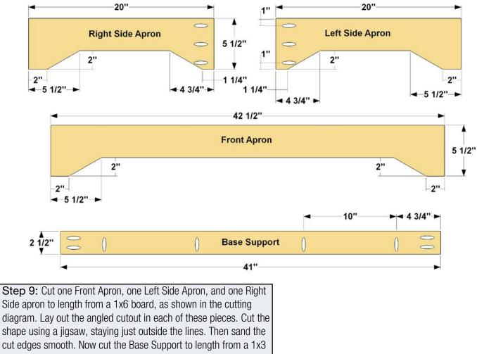
board. Drill pocket holes in all of these parts where shown.
