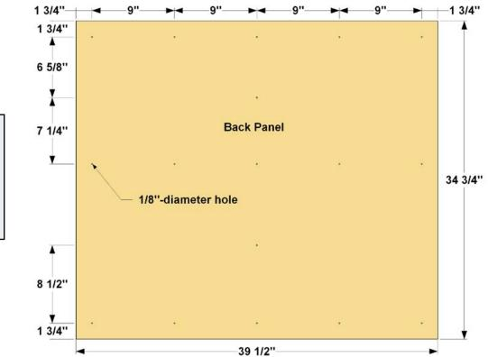
Step 17: Cut a Back Panel to size from 1/4" plywood, as shown in the cutting diagram. Then lay out and drill 1/8 holes where shown. These will be used for screws that will attach the back panel later.
