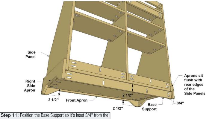
Step 11: Position the Base Support so it's inset 3/4" from the rear edge of the Side Panel, and then secure the Base Support with 1 1/4" coarse-thread pocket hole screws. Next, slide the apron assembly in place so it hangs down 2 1/2" below the Bottom Panel. You can use a scrap of 1x3 to do this. Make sure that the Side Aprons are flush with the lower edge of the Base Support, as well. Then attach the apron assembly using 1 1/4" coarse-thread pocket hole screws.
