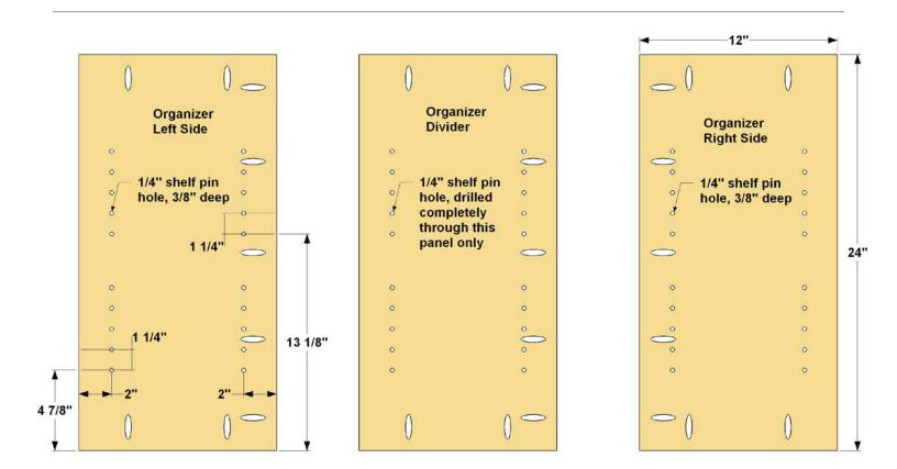
Step 16: Cut one Left Organizer Side, one Organizer Divider, and one Right Organizer Side to size from 3/4" MDF. Then you need to drill shelf pin holes in these parts. Before you do this, mark the bottom edge of each piece so you get all of the holes positioned correctly. Note that the Divider needs holes in both faces. After you drill the shelf pin holes, drill pocket holes, as shown, with your pocket hole jig set up for 3/4" material.
