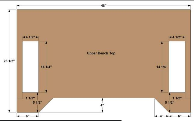
**Step 6:** Cut one Upper Bench Top to size from 3/4" MDF, as shown in the cutting diagram. Then lay out and cut the recess along the front edge using a jigsaw. Next, lay out and create the tray openings. Start by drilling a hole at each corner, then cutting along the lines with a jigsaw.
