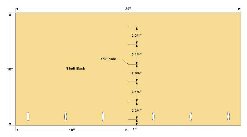
Step 11: Cut a Shelf Back to size from 3/4" MDF, as shown in the cutting diagram. Then drill pocket holes where shown. After that, you need to drill a row of holes through the Shelf Back, as shown. These will be used for screws that attach the Shelf Dividers.
