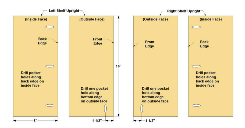
Step 10: Cut two Shelf Uprights to size from ¾" MDF, as shown in the cutting diagram. Then drill pocket holes where shown with your pocket hole jig set up for 3/4" material. Note that you need to create a "matched pair" of uprights. You'll drill pocket holes along the back edge of each one on the inside face. Then you need to drill one pocket hole in the outside face of each upright, as shown.
