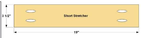
**Step 2:** Assemble the bench ends by attaching the Short Stretchers to the Legs using 2 1/2" pocket hole screws, as shown.
