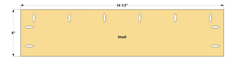
**Step 9:** Cut three Shelves to size from 3/4" MDF, as shown in the cutting diagram. Cut three Shelf Dividers while you're at it. Then, with your pocket hole jig set up for 3/4" material, drill pocket holes in the Shelves, as shown.
