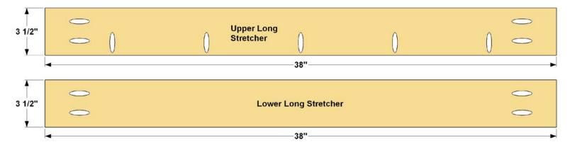
**Step 3:** Cut five Long Stretchers to length from 2x4 boards, as shown in the cutting diagram. With your pocket hole jig set up for 1 1/2" material, drill pocket holes in three of pieces to create three Upper Long Stretchers. Then, create two Lower Long Stretchers by drilling those pocket holes where shown.
