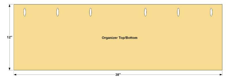
**Step 15:** Cut one Organizer Back, one Organizer Top, and one Organizer Bottom to size from 3/4" MDF, as shown in the cutting diagram. With your pocket hole jig set up for 3/4" material, drill pocket holes in the Organizer Top and Bottom as shown.
